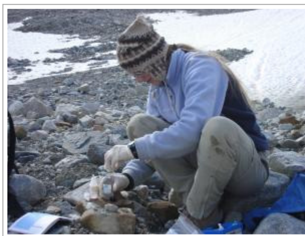
The Winkler method is done by noting a color change when titrating a fresh water sample. Photo provided by Monica Bruckner.
