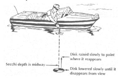
The Secchi disk is used to measure how deep a person can see into the water. It is lowered into the lake by unwinding the waterproof tape to which it is attached and until the observer loses sight of it. The disk is then raised until it reappears. The depth of the water where the disk vanishes and reappears is the Secchi disk reading. The depth level reading on the tape at the surface level of the lake is recorded to the nearest foot.
